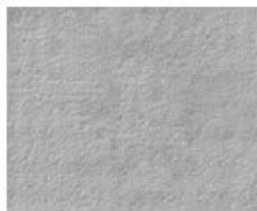
CSP 3 – Jateamento leve 965,2 \mu\text{m}^*
