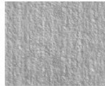
CSP 4 – Jateamento leve/médio 1270 \mu\text{m}^*
